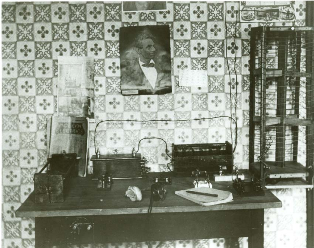
Caption: Tom Appleby commented, "This is my homebrew station in 1908. Call "HN" but listed in the 1909 Blue Book of the Wireless Association of America, as "HNM". Note the antenna helix on the right, then the rack of 4 x 5 glass photo-plate condensers, the 1" spark coil with ball spark gap across the secondary, the single receiver head phone with a pad for the other ear, the two slide tuning coil made from a rolling pin, the electrolytic detector in front of the spark coil, it had leverage action to raise the point of the Wollaston wire from the acid in the platinum cup and last if not least, the copy of Modern Electrics magazine bearing the date, if your eyes are good, February 1908, or it could have been 1909 as it is close to the new year. But the outfit was in operation in 1908."
