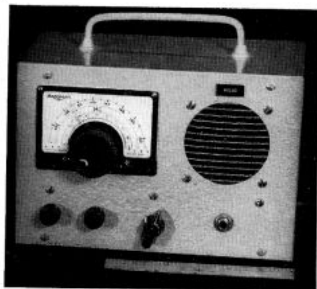
The club-project 2-meter portable station described by W9LUO. Size may be judged from the 6-inch scale at the lower right. Power supply is a separate unit, and may be arranged to suit user's requirements.
