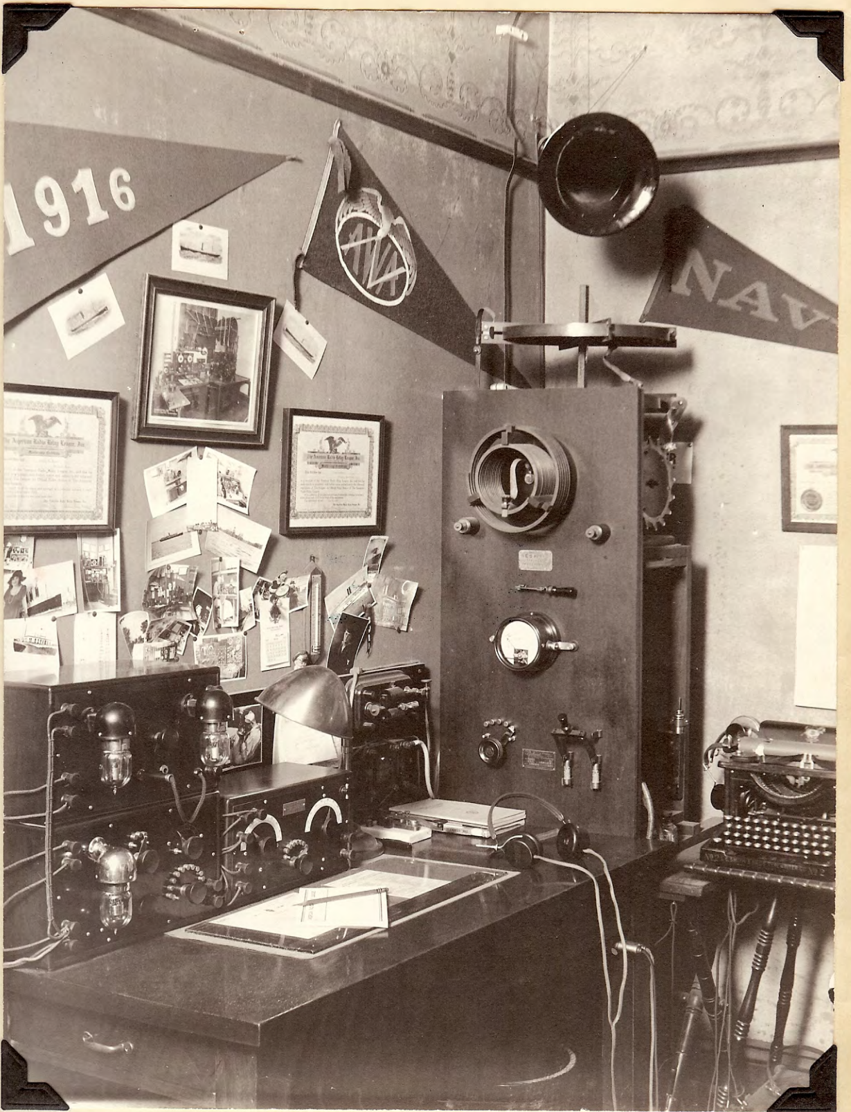
1/2 K.W. SPARK TRANSMITTER, "3CS" LOCATED AT 931 EDGEWOOD AVE., TRENTON FROM 1919 T 1922. EQUIPMENT ALL HOME BUILT, EXCEPT UNITED WIRELESS MARBLE BASE KEY, THERMO-ANTENNA AMETER, AND MICA DIAPHRAM "BALDWIN" PHONES. THE RECEIVER IS A REGENERATIVE TYPE, 150-700 METERS, WITH MOORHEAD AUDION DETECTOR AND 2-STAGE
