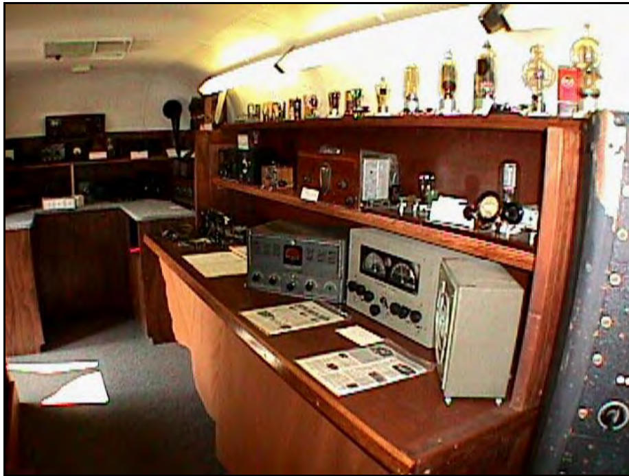
Various 1924-1939 ham radio stations, both homebrew and commercial. The earlier tube gear and Spark transmitters are in the rear.
